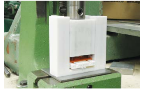
An operator modified 350 connectors in about an hour on this toggle press.
