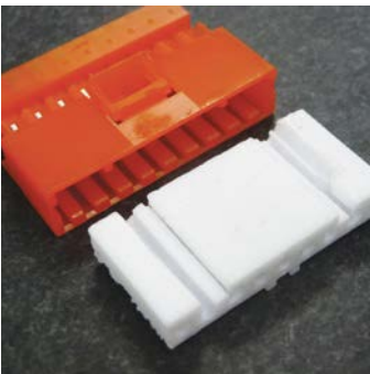
The white FDM piece supported each connector during punching.
