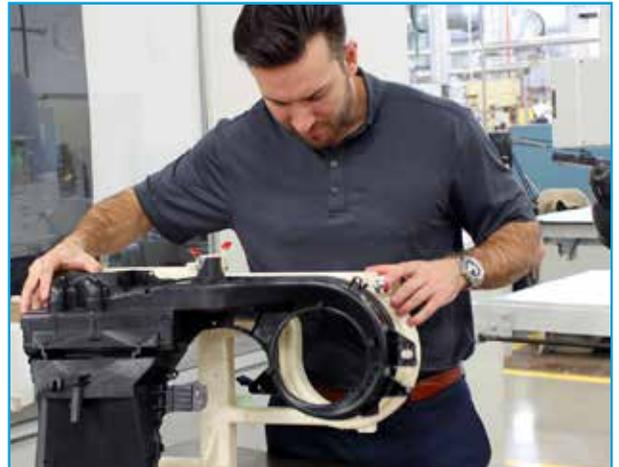
In less than a week, MAHLE had a redesigned, dimensionally accurate and stable part delivered to them from across the world – a process that would have taken 4 to 5 weeks with conventional manufacturing. Thanks to part consolidation, the fixture had a continuous and smooth mating interface, which could only be replicated in a metal fixture at a considerable cost, saving MAHLE thousands by using 3D printing instead of CNC machining.
