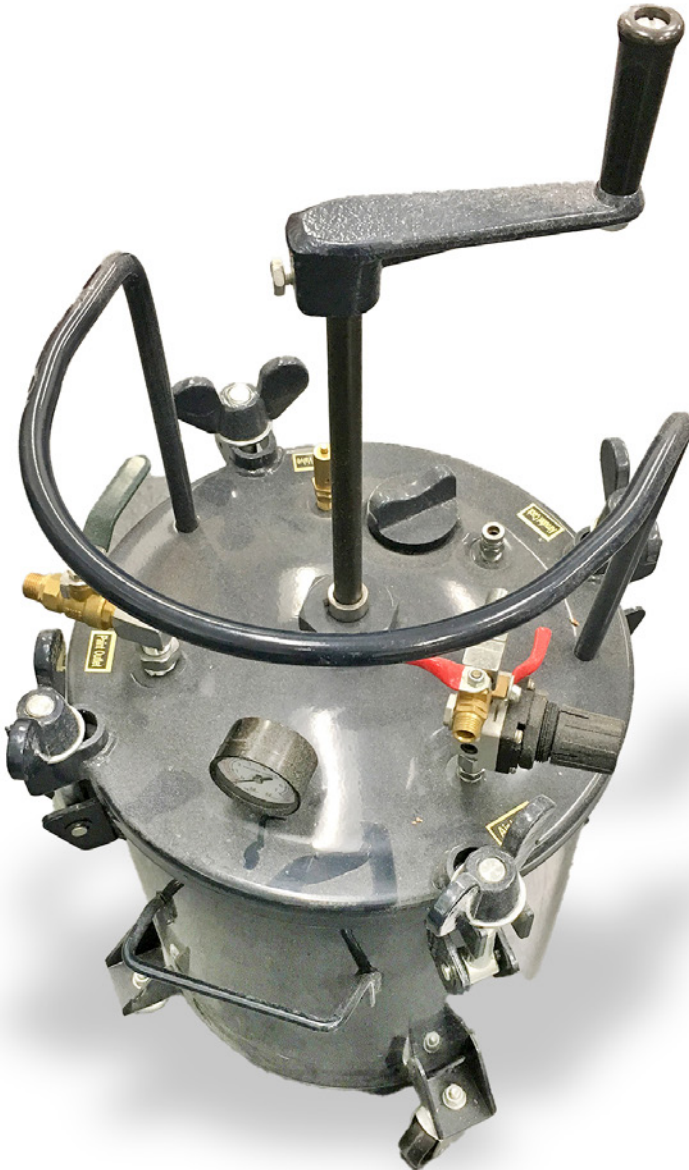
Figure 26: Vacuum impregnation can be performed using small vacuum pots or large industrial impregnation centers.
