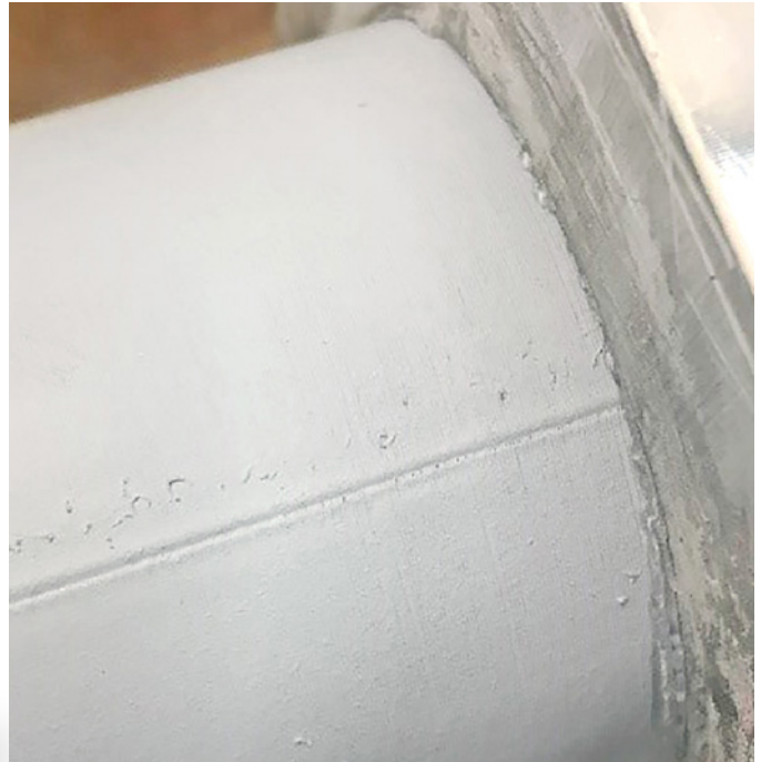
Figure 27: Standard aerospace or automotive paints formulated for plastics can be used to seal FDM ducting for low-pressure applications.
