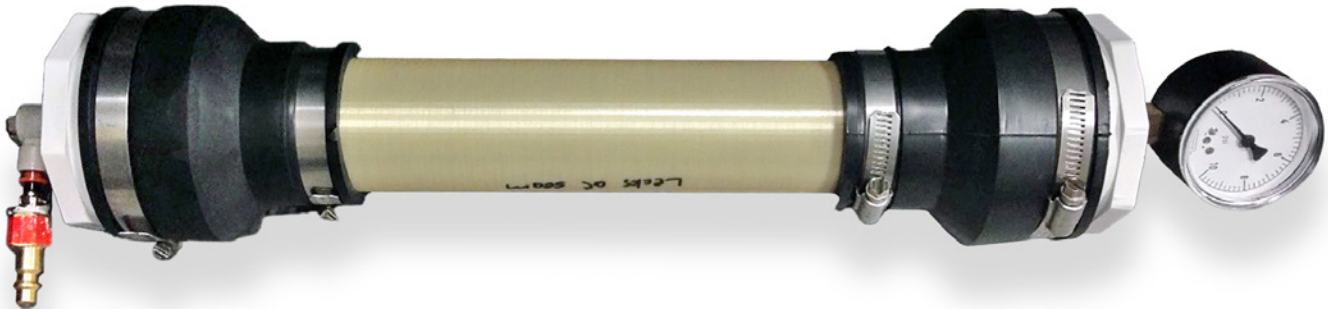
Figure 24: FDM parts exhibit a process-induced porosity that is undesirable in ECS ducting. If the pressure loss incurred from the presence of the porosity is not tolerable, use a secondary process to seal the parts.
