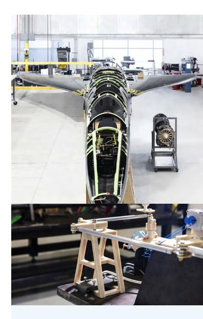
Boom Supersonic used 3D printed flight control test rig tooling for its XB-1 supersonic jet. The printed tools resulted in a 90% cost and lead time savings over conventionally produced tooling.
