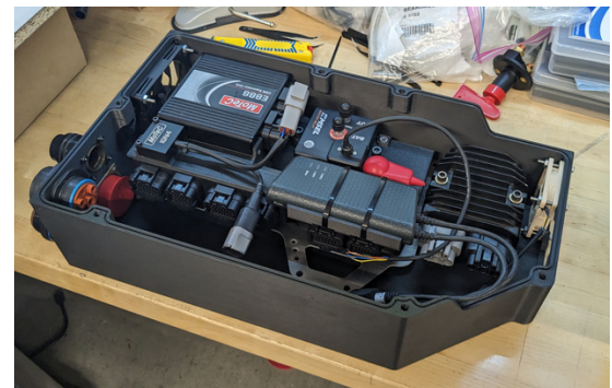
FDM Nylon 12CF Electronics Enclosure
