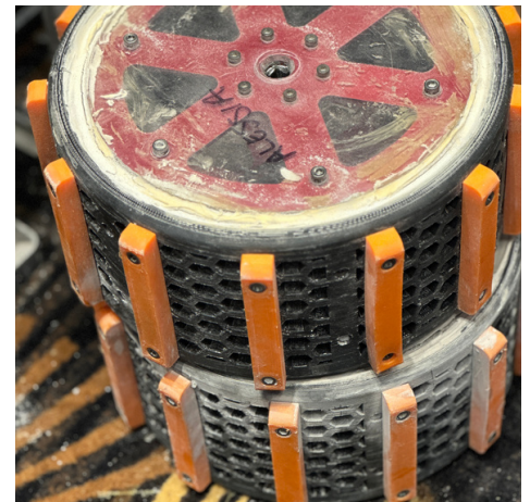
Wheel assembly made using FDM TPU 92A
