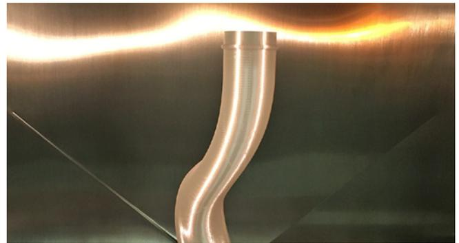
A duct built in a vertical orientation to improve sealing and surface finish.
