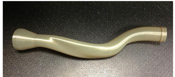
A finished custom duct showing the complex shapes made possible with FDM technology.
