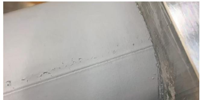
Standard automotive or aerospace paint can be used as a sealant for low-pressure applications.
