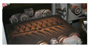
Figure 31: Cope side of sand mold for window handle.
