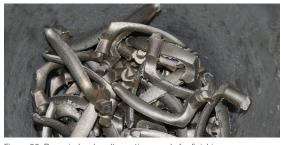
Figure 36: Raw window handle castings ready for finishing.
