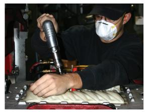
Figure 29: Mount matchplate in automated molding machine.
