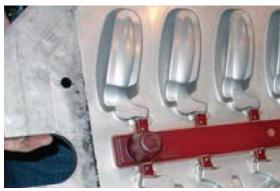
Figure 2: Machined aluminum matchplate.
