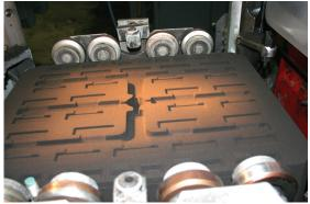
Figure 3: Flaskless, green sand cope.
