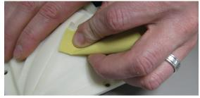
Figure 25: After support removal, smooth pattern surfaces.
