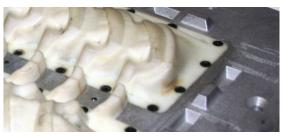
Figure 12: Matchplate blank incorporates a thick "rib" between inserts for stiffening.
