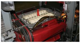
Figure 30: Matchplate in automated molding machine.
