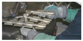
Figure 35: Cut off gates.
