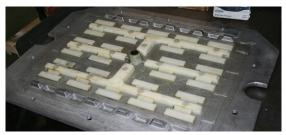
Figure 13: Split pattern matchplate. FDM patterns mount flush to each side of blank.
