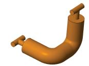
Figure 16: CAD model of core with core plugs.
