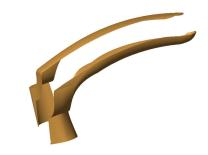
Figure 7: Split the CAD model along the parting line and separate the halves by the thickness of the matchplate blank.
