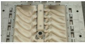
Figure 27: Complete matchplate (drag side shown) with two pattern inserts and removable gate/runner system.
