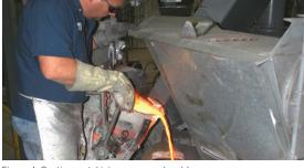
Figure 4: Casting metal into green sand mold.
