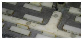
Figure 15: Making gating and runner system as a separate piece; it may be interchanged with alternate configurations.
