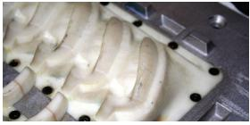
Figure 26: Mount (bolt) FDM insert to machined matchplate blank.
