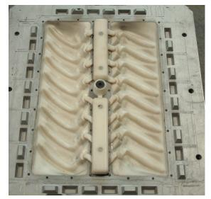
FDM matchplate insert with interchangeable gate and runner system.
