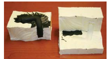
Figure 9: A urethane casting, with the soluble core, prior to extraction from the RTV mold. The black material on the mold's surface is flash from the casting operation.
