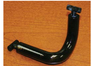
Figure 4: A soluble core for the radiator hose.
