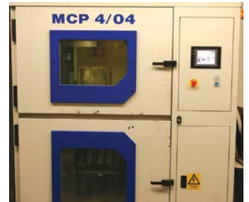
Figure 8: The two-part urethane and RTV mold are placed in the automated vacuum casting machine.
