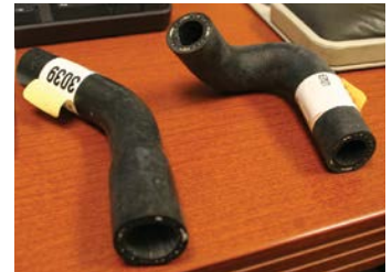
Figure 1: These hoses are examples of parts that need soluble cores since the RTV tool cannot be extracted from the internal passage.
