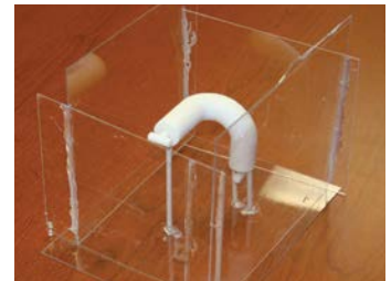
Figure 5: The pattern is mounted on dowels and attached to the floor of the mold box.
