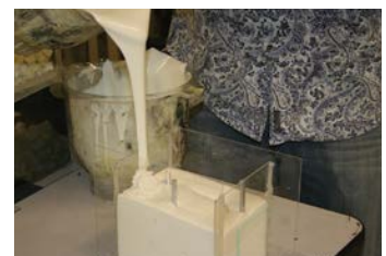
Figure 6: The RTV rubber is poured into the pattern and then allowed to cure.
