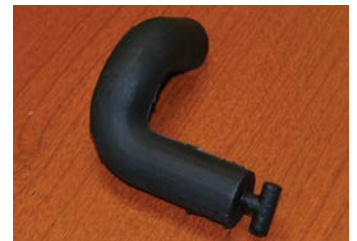
Figure 10: Finished hose part with soluble core in.
