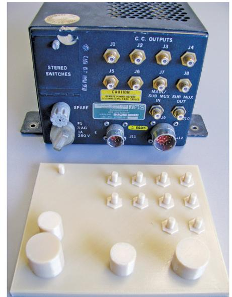
Figure 7: FDM surrogate with simplified interface connections.
