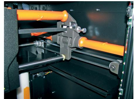
Figure 13: Color-code surrogates to indicate “Remove during installation.”
