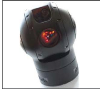
Figure 90: Production assembly utilizing FDM end-use parts (ABS-M30).
