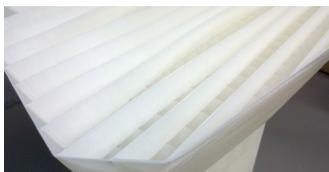
Figure 68: Support tower with wide air gaps to decrease build time.
