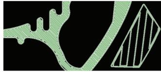
Figure 70: Default Sparse support toolpaths (right).
