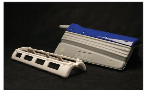
Figure 9: Final product next to FDM component. Material properties allow for MRI functionality (polycarbonate).
