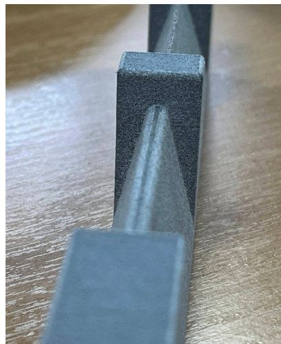
Radius applied to the edge, more robust
