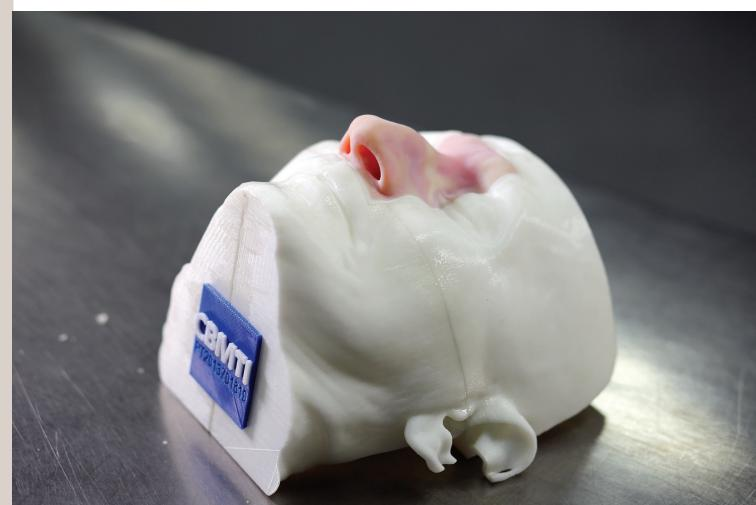
The simulation section is installed in a reusable 3D printed head fixture
