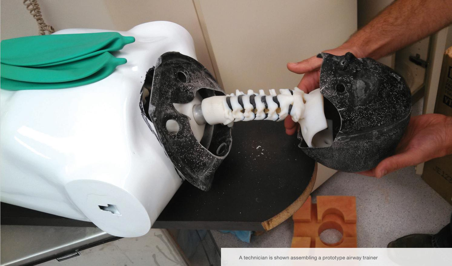
A technician is shown assembling a prototype airway trainer
