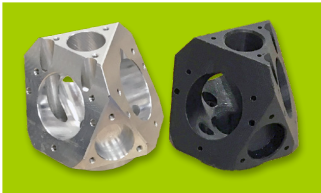
Figure 2: CNC (aluminum) on the left, 3D printed (plastic), right.
