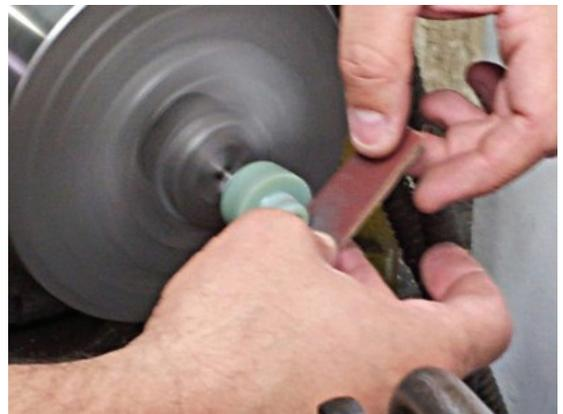
Figure 11: Finishing process of mold component.
