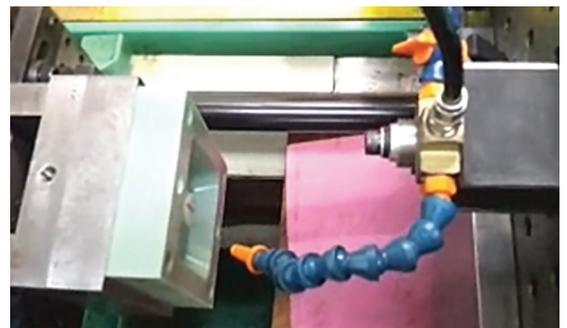
Figure 14: Cooling fixture mounted on the mold. As the mold opens, pressurized air is applied to the surface for a predetermined time.
