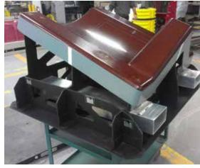
Figure 8. Speaker box FRP mold.
