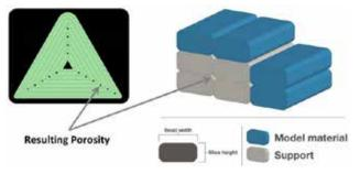
Figure 3. This cross-section of FDM tool paths illustrate the inherent occurrence of porosity (from Stratasys Insight software).
