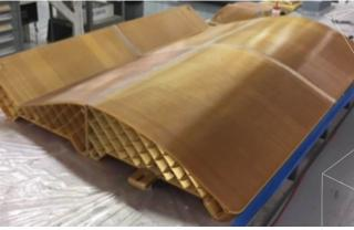
Figure 15. Assembled 4-piece FDM cabinet headliner lay-up mold.
