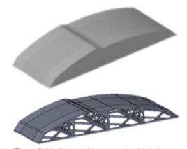
Figure 5. Medicine cabinet panel mold designs. Sparse style (top) and shell style (bottom).
