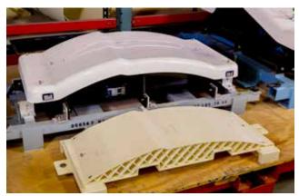
Figure 7. View of the FRP machining fixture (top) next to the FDM machining fixture (bottom).
