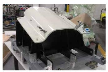
Figure 11. FRP machining fixture for the speaker box panel.
