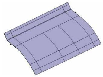
Figure 13. CAD rendering of the cabinet headliner panel.
