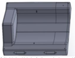
Figure 10. Updated mold design for the speaker box panel for improved handling.
