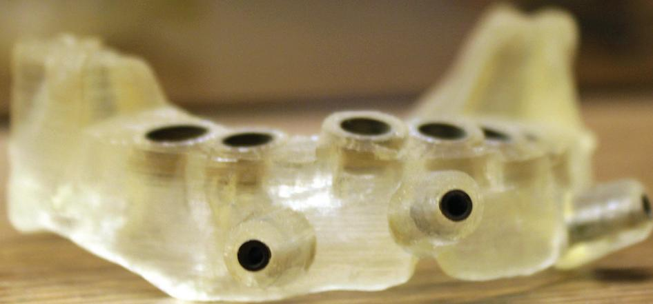
3D printed dental guides to accurately locate implants
