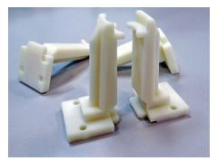
3D printed handling fixture in VeroWhite material. Installed on a robot, this manufacturing tool enables the team to lift the caps on the rigid packaging during production.
