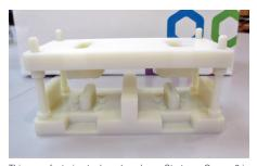
This manufacturing tool produced on a Stratasys Connex3 is used to verify the thickness of the final production part.
