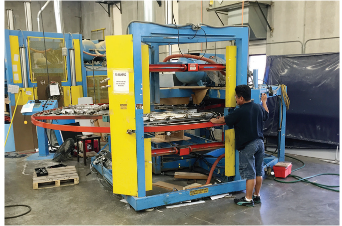
Figure 28 – FDM tooling works with the same thermoforming equipment, processes and procedures used with traditional tooling methods.
