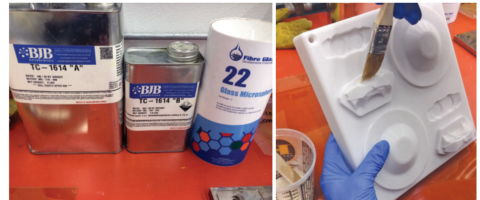
Figure 26 - Removing porosity in some regions of the tool by sealing with epoxy may be required to promote flow of the sheet over these surfaces.
