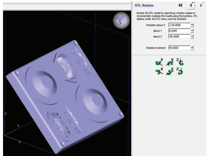
Figure 15 - The rotation menu in Insight allows for unique orientations to be achieved by incrementally rotating the .stl by a specified angle about the X, Y, and Z axis.
