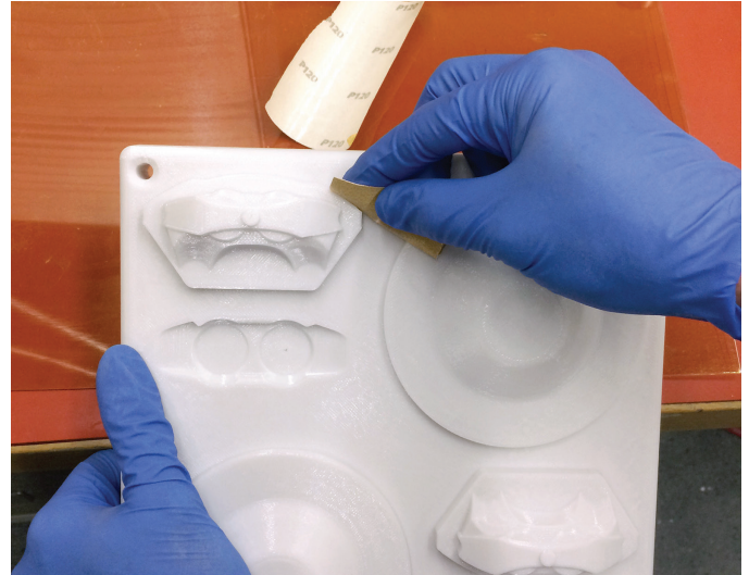
Figure 25 - Improving the surface finish of the tool will improve the surface finish of the formed parts.
