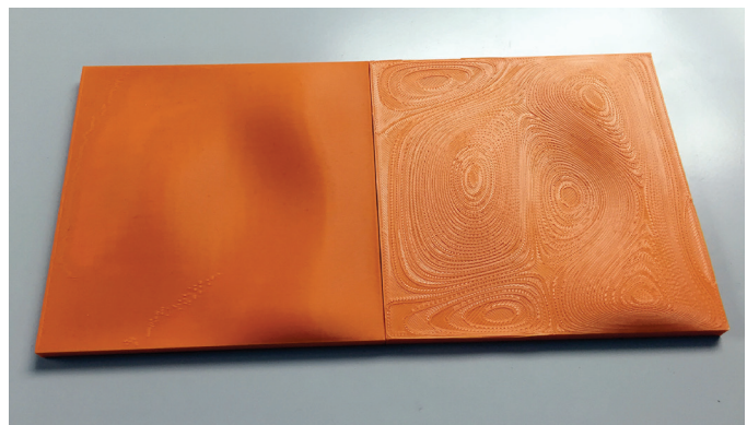
Figure 12 - A tool with gradually sloped surfaces will have a better surface finish when built in a vertical orientation (left) and may become stair-stepped when built flat due to the FDM layering process (right).
