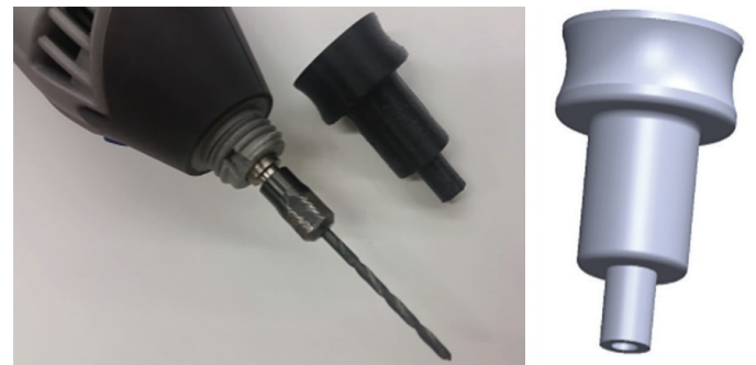
Figure 32 - The head of the rotary tool and attachment to guide the cut.
