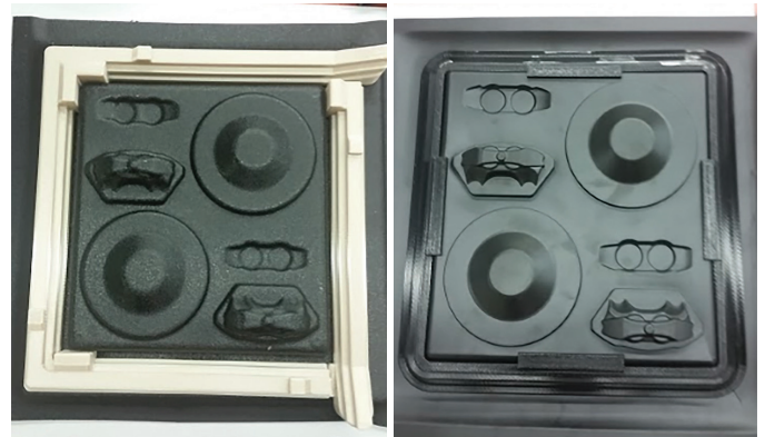
Figure 39 - Finished trim tools for an oscillating cutter (left) and rotary cutter (right).
