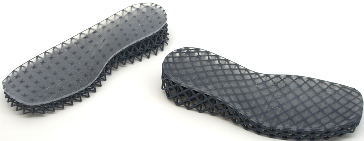
DManD researchers created multi-material soft-lattice structures for this footwear prototype using a custom design, analysis and slicer tools to spatially control stiffness and non-linear
