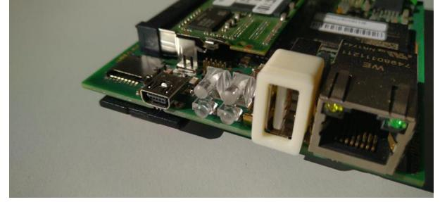
3D printed prototype of a USB port
