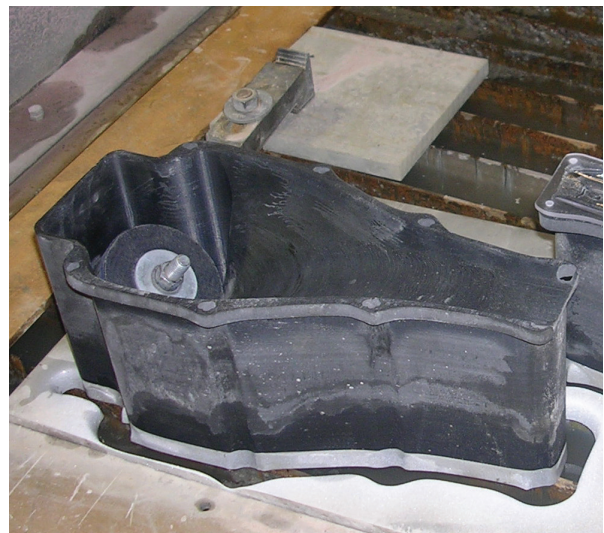
Top NASCAR team, Joe Gibbs Racing, uses FDM to make fixtures, some of which have been in service for more than two years and have cut lead time and expense by an average of 70 percent.
