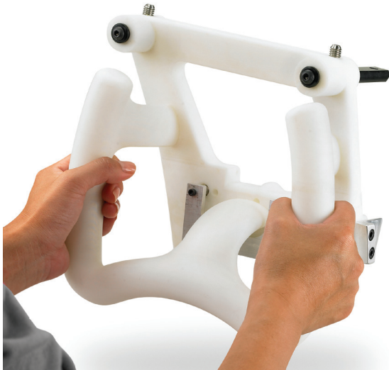
Using FDM, BMW prints jigs and fixtures that would not be possible with conventional machining and fabrication. AM allows them to be easier to use and more functional.
