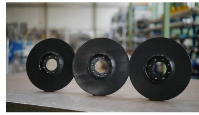
For the impeller, 3D printing has significantly reduced lead times by up to 50% compared to traditional metal machining.
