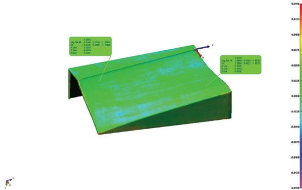
Figure 5 – 3D scan data for a UAV fan blade (shell style) tool after 10 thermal cycles with color map comparison to the 3D scan data for the same tool prior to cycling. Dimensions are in inches.
