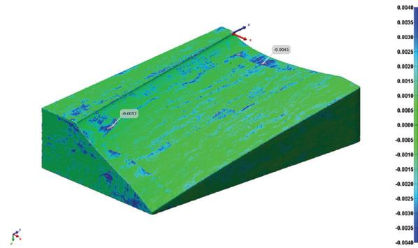
Figure 6 – 90 thermal cycles before vs. after dimensional comparison.
