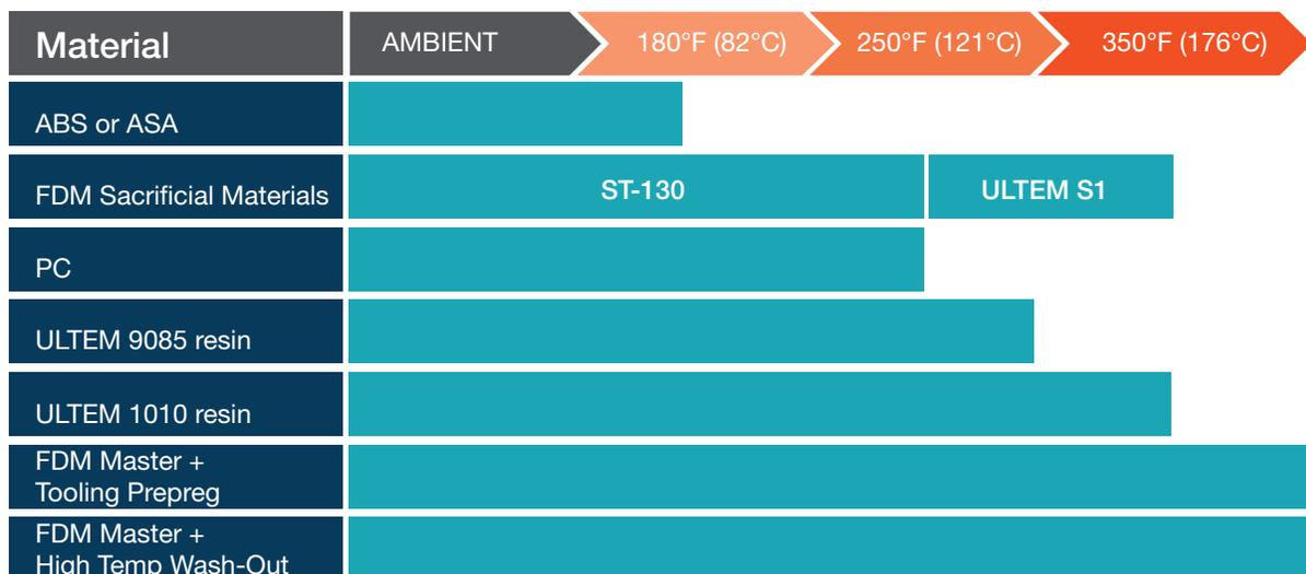
Figure 1 – Temperature capabilities of FDM materials.
