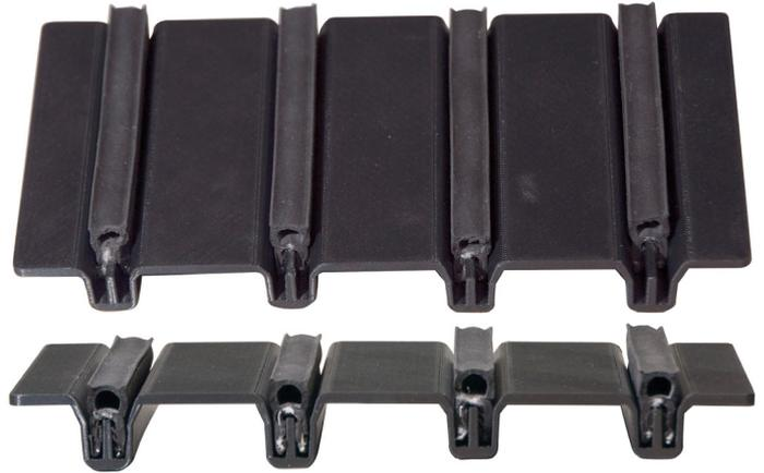
This FDM part (top and side view) allows testing of four variations of a groove that mates with a rubber seal. The finished HVAC system housing (below) features three FDM parts.
