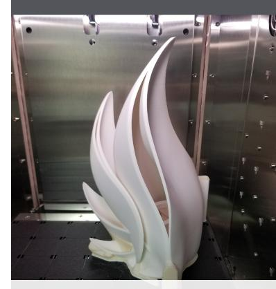
A student lamp project, printed on the F370 FDM printer.
