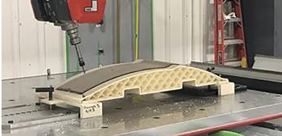
Figure 7. Composite panel being machined using the FDM fixture.
