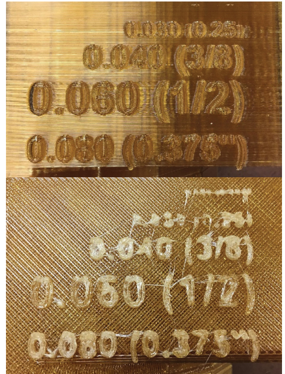
Figure 3. Protruding text printed in the vertical orientation (top) and horizontal orientation (bottom).
