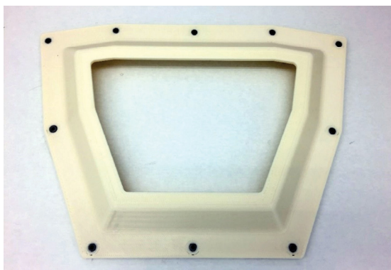
Figure 5. Trim and drill jig printed with ASA.
