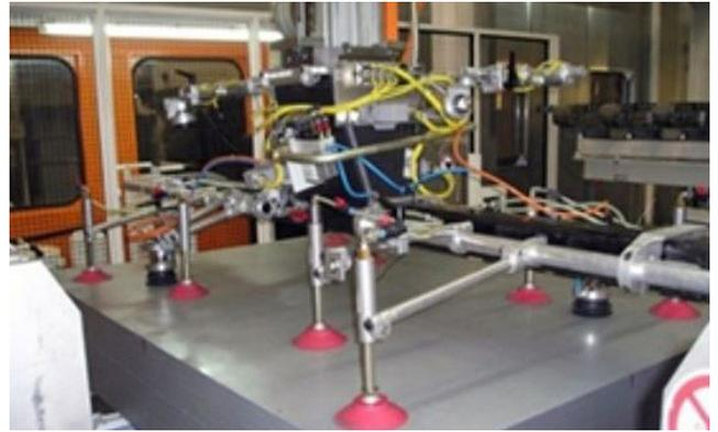
Lifting tool used to move sheet metal blanks.
