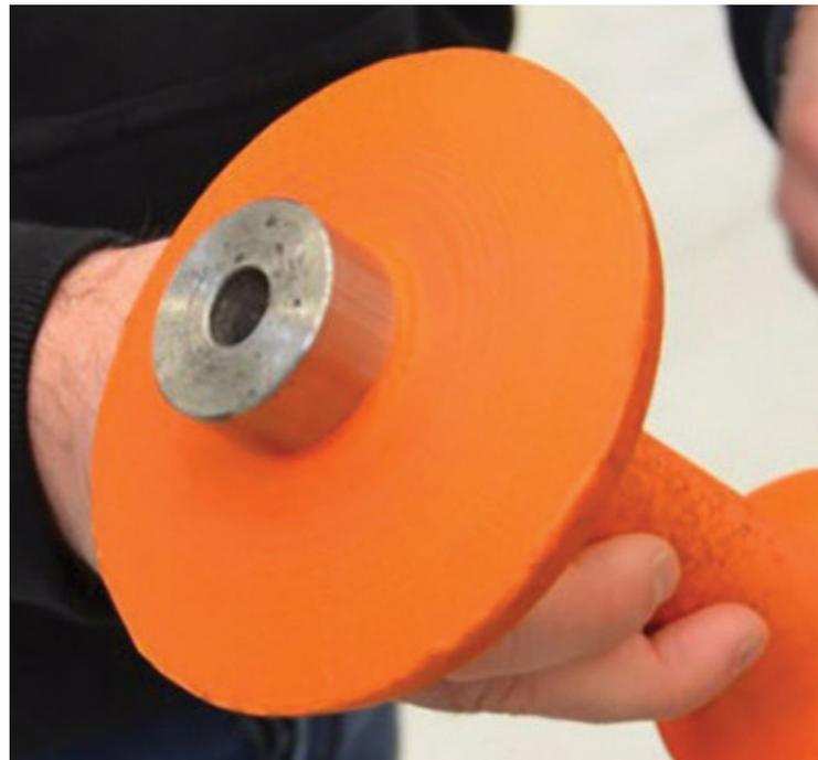
This lightweight tool is used for punching operations.
