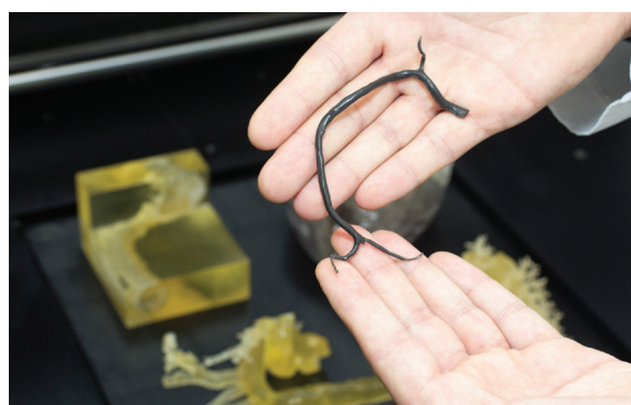
The Objet350 Connex's rubber-like material is ideal for prototyping arteries.
